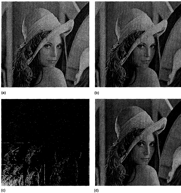
Figure 2. FAWAV output: a noisy Lena (Gr 1), a denoised Lena (Gr 2), significance map from thresholded transform used in denoising (Gr 3), and the original Lena (Gr 4).
