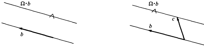
Figure 4.1 (left). The action of a 2-form \Omega on the vector b yields a 1-form \Omega \cdot b . The data in this figure completely specifies \Omega in two dimensions.
