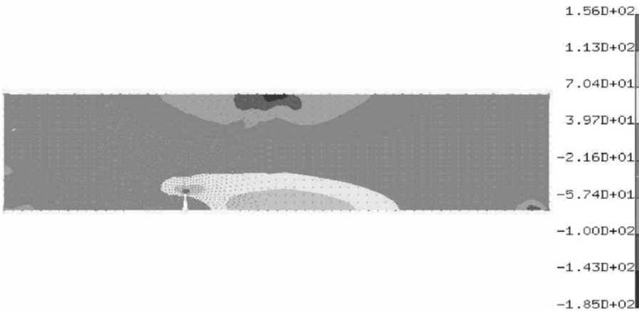
FIGURE 6.10. Stress ( t_{xx} in GPa) distribution of a three-point bending beam with edge crack.
