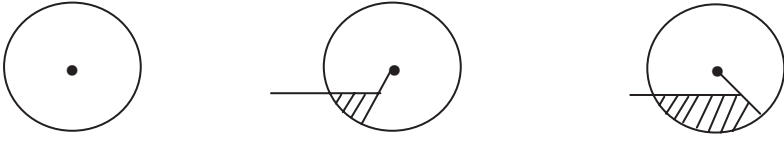
(a) no crack in the domain of influence (b) the presence of a crack (c) crack growth
