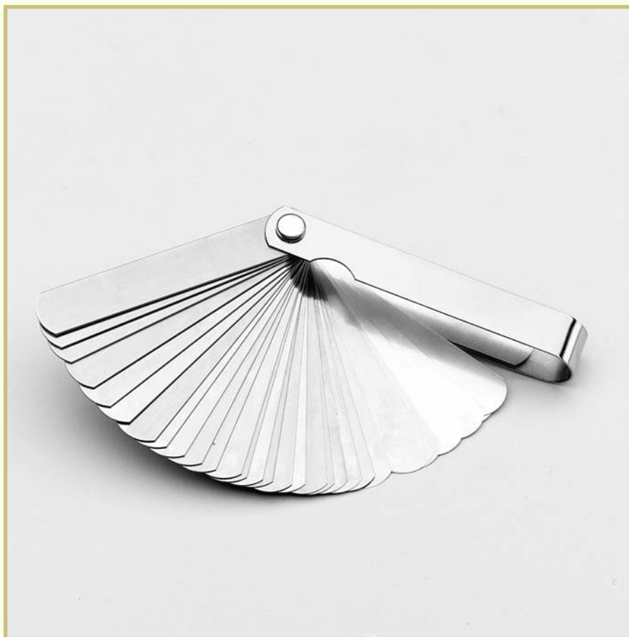
FIGURE 45 —A blade-type feeler gage is made up of a selection of metal blades that spread open like a fan. Each blade is marked with its thickness, both in thousandths of an inch and in millimeters.
