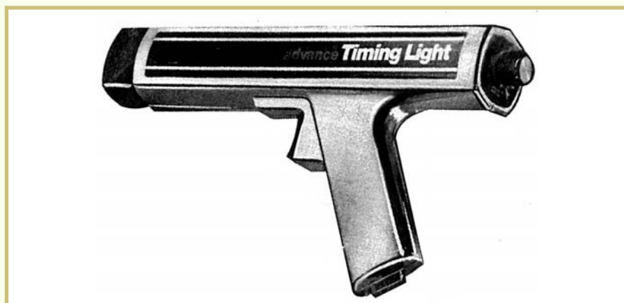
FIGURE 49 —The timing light shown here is used to test ignition timing with the engine running. The timing light will flash each time the spark plug fires.
