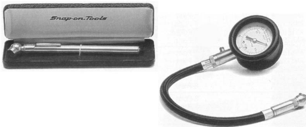
FIGURE 52 —Two common types of tire pressure gages are shown here. (Courtesy of Snap-On Tools Company, Copyright Owner)
