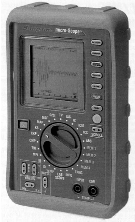
FIGURE 51 —A scan tool allows the technician to connect into a vehicle's electronic system and scan or monitor the signals produced by the system. (Courtesy of Snap-On Tools Company, Copyright Owner)
