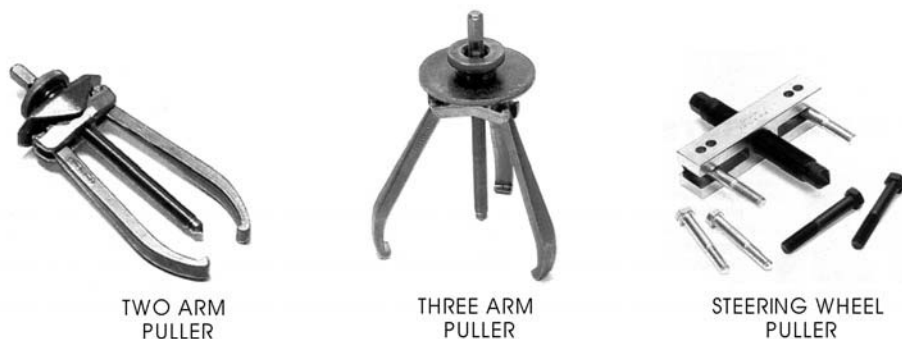
FIGURE 32—A variety of different pullers are illustrated here. (Courtesy of Snap-On Tools Company, Copyright Owner)
