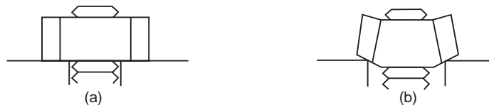
Figure 6.2 Schematic illustrating (a) proper nut seating and (b) improper nut seating due to an oversize bolt hole.
