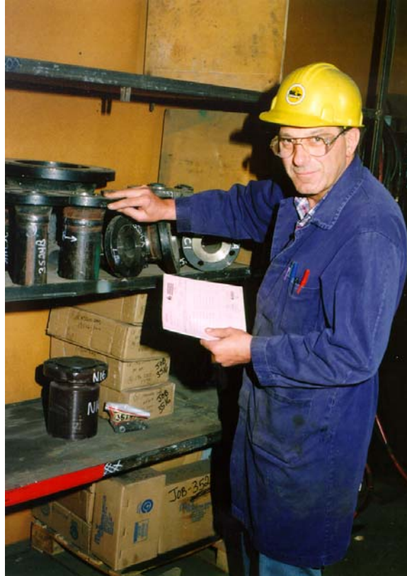
Figure 11.1 This inspector is checking mill certificates against permanent die stampings on the fittings to be used for pressure vessel fabrication.
