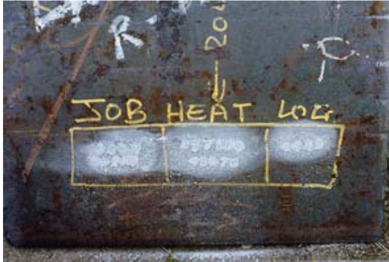
Figure 4.2 Die stamp identification marks on a section of carbon steel plate that has been formed into a vessel shell.
