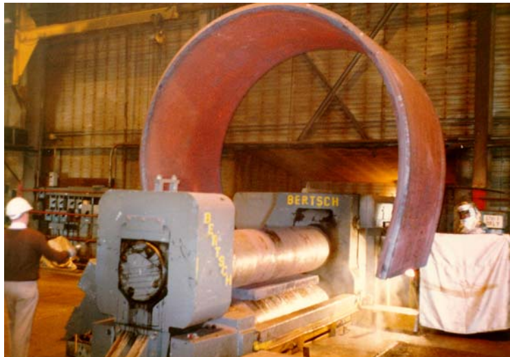
Figure 6.1 A 4\frac{1}{2} inch (115 mm) thick plate being hot roll formed into a cylindrical section for a pressure vessel.
