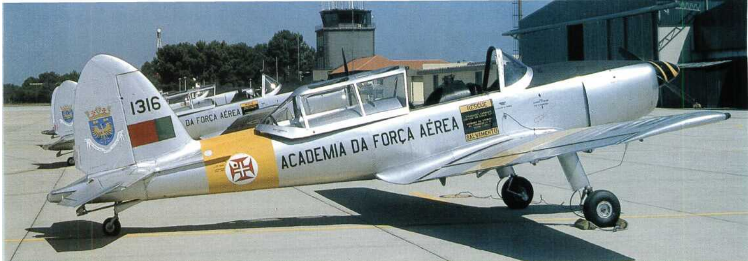
Portugal is one of the few countries that still uses the DHC-1 Chipmunk. The Portuguese Air Force Academy uses the type - with the original engines replaced by Lycomings - for air experience flights and as glider tugs. RUI FERREIRA
