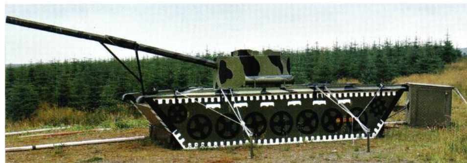
In addition to the various radiating threat systems, which can be located virtually anywhere in the range area, there are also large numbers of locally-made mock-up systems, representing tanks and armoured fighting vehicles. For greater realism, these can be provided with a heat source inside the body of the vehicle to reproduce an appropriate infra-red signature.
