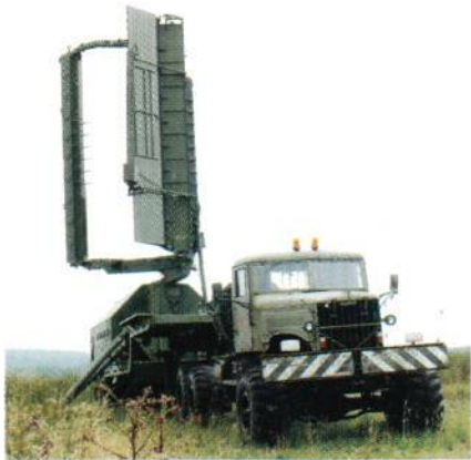
This non-operational Tin Shield 3D E/F-band target acquisition radar is mounted on high ground near the old mock airfield at Prior Lancey, with an associated control van alongside. Yet another example of the range's visual realism, it adds to the value of the electronic threats from real systems, emulators and simulators.
