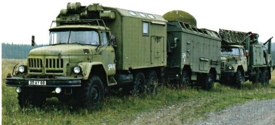
Adding further realism to the military hardware at Spadeadam is a 'convoy' of defunct Russian equipment, which includes a number of electronic box-body vehicles, including this King Pin trailer-mounted jamming system. Although no longer functional, the vehicles represent the type of equipment still in use in potentially hostile theatres and are a valuable adjunct to the real electronic threats.
