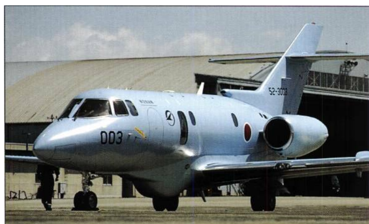
Above: Heavily-modified Hawker 800s (BAe 125-800s) were acquired from 1995 for maritime patrol and SAR duties. A total of 27 (U-125As) has been ordered. A navaid calibration version of the U-125 is also in use.
