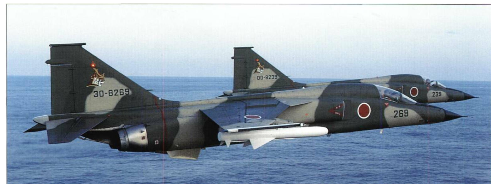
Below: These Mitsubishi F-1s of 3 Hikotai (3 Kokudan) are armed with the F-1's primary weapon, the Type 80 ASM-1 anti-ship missile. The missile entered service in 1983 and has a 50-km (31-mile) range with a 150-kg (330-lb) HE warhead.
