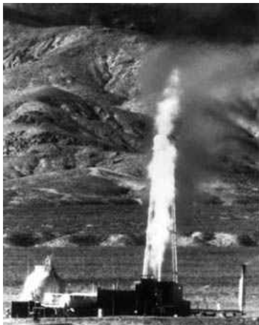
NERVA nuclear rocket under test. (Smithsonian Institution Photo No. 75-13750)
