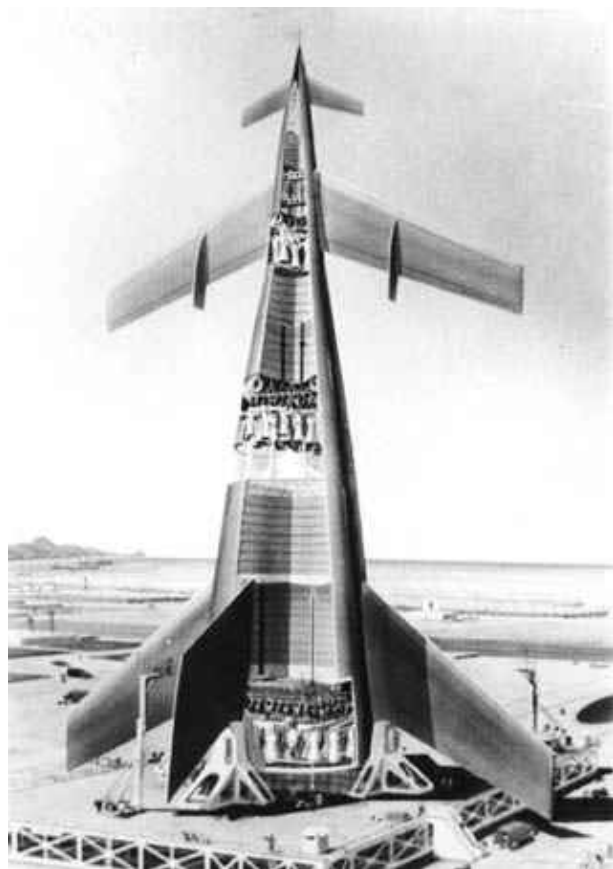
Cargo rocket of the Collier's series, with winged upper stage. (Art by Rolf Klep; courtesy of Ron Miller)
