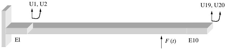
Figure 1. Fixed-free beam element numbers and nodal dofs for simulation.
