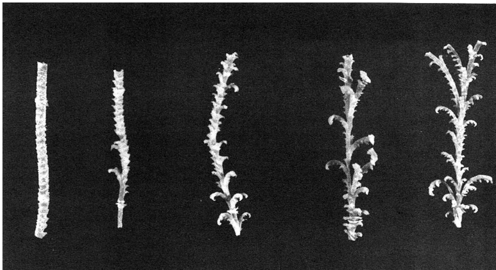
Figure 4.15. Instability of flow leading to disruption of a stream: transition from left to right corresponds to increase of velocity (shear rate).
