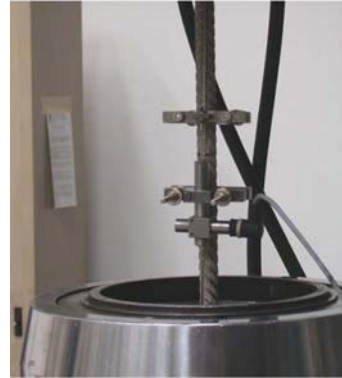
Fig 2. Elongation test apparatus.
