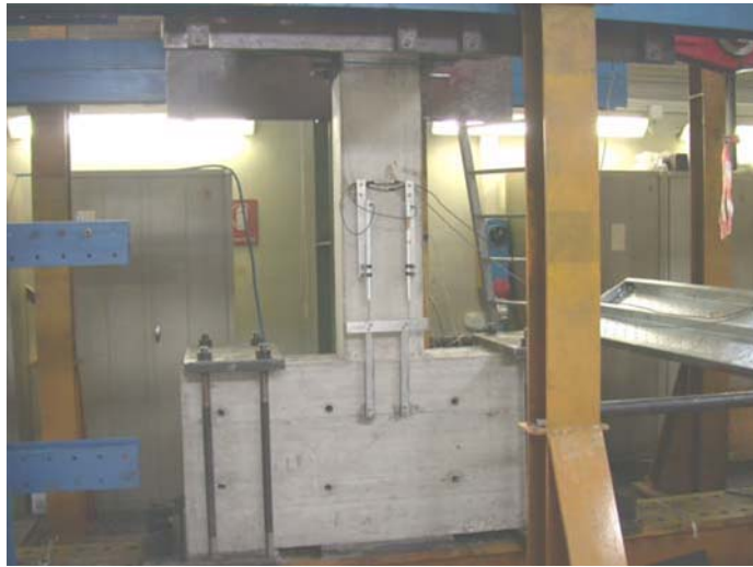
Fig. 12. Test rig and the column prototype.
