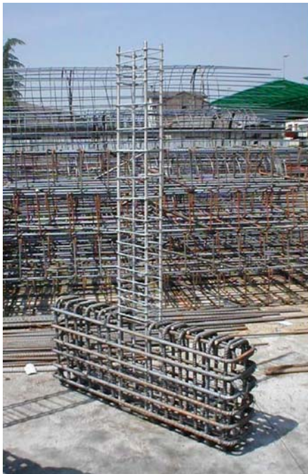
Fig. 11. Steel reinforcement of the column prototype.
