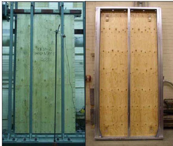
Figure 1. Typical 1220×2440 mm shear wall test specimens.
