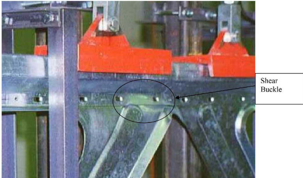
Fig. 7. Typical shear failure.
