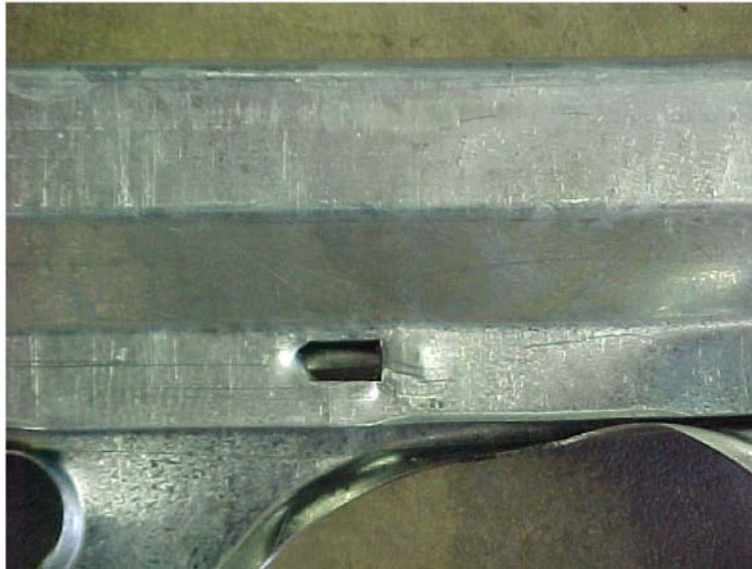
Fig. 5. Typical clinch failure.
