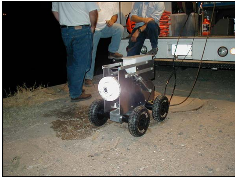
Figure 6. Second generation wheeled inspection robot with gpr
