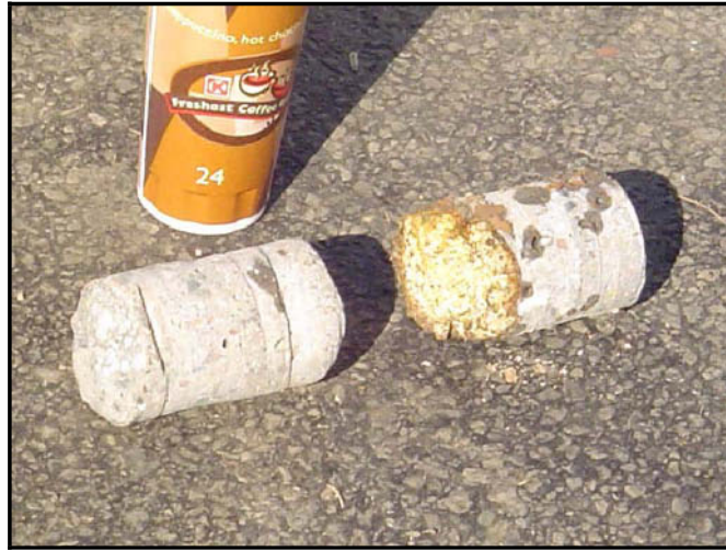
Figure 9. Core samples from 750 mm concrete pipe section
