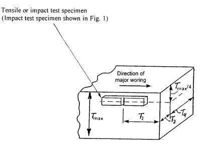
Note—For material with thickness T greater than 2 in. [50 mm],  $T_2=T_3=T_4 \ge T_{max}T_{max} =$  maximum heat treated thickness FIG. 1 Test Specimen Location for Quenched and Tempered Forgings areas subjected to magnetic particle test to assure freedom from cracks unless the welded areas are completely removed by subsequent machining.
