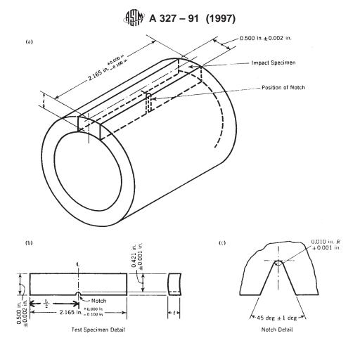
In Diagrams (a) and (b) the symbol t is for the pipe wall thickness. Permissible variations for  $\frac{1}{2}$  shall be  $\pm 0.040$  in.
