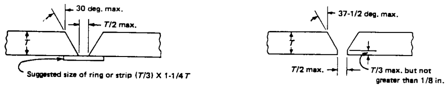
FIG. 5 Joint Preparation
