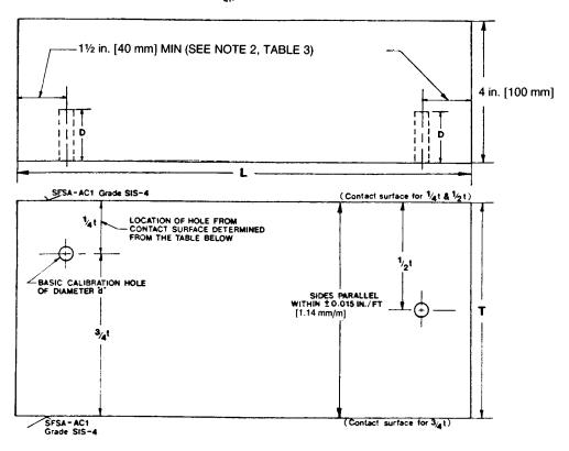
L = length of block determined by the angle of search unit and the vee-path used,
