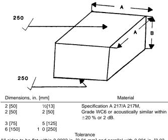
All sides to be flat within 0.0002 in. [0.01 mm] and parallel with 0.001 in. [0.03 mm].
