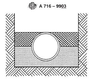
NOTE 1—Pipe is bedded to its centerline in compacted granular material with a minimum of 4 in. (102 mm) under the pipe. Compacted granular or select<sup>A</sup> material is used to the top of the pipe. (Material is compacted to approximately 90 % Standard Proctor in accordance with AASHTO Standard T-99.)
