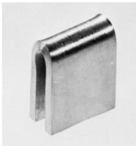
FIG. 10 A Bent Copper–Copper Sulfate–Sulfuric Acid Test Specimen
