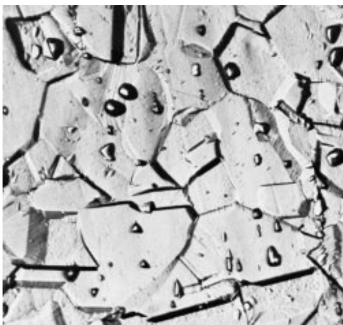
FIG. 1 Step Structure (500 \times ) (Steps between grains, no ditches at grain boundaries)
