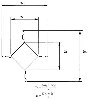
FIG. A1.1 Hardness and Toughness Calculation
