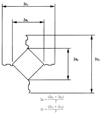
FIG. A1.1 Hardness and Toughness Calculation
