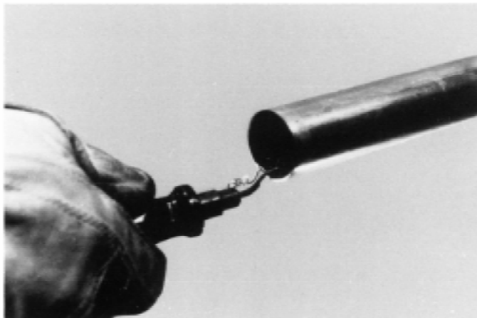
FIG. 5 Reaming: Deburring Tool
