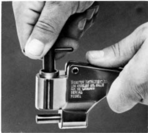
FIG. 4 Adjusting Load on Load Spring
