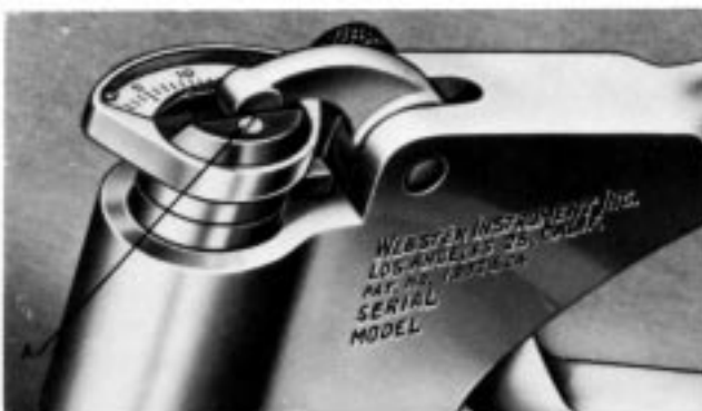
FIG. 3 Zero Adjustment Screw, A (indicated by arrow)
