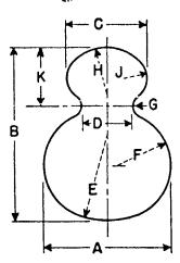
NOTE-For dimensions E, F and H the dimensional tolerance is ±0.016 in. (0.406 mm); for dimensions G and J the dimensional tolerance is ±0.008 in. (0.203 mm).
