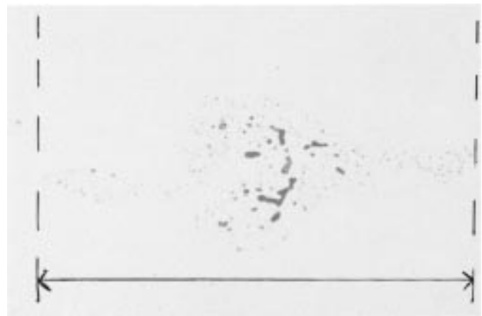
FIG. 3 Example of a spotty oxide inclusion. The maximum Feret’s diameter is indicated.
