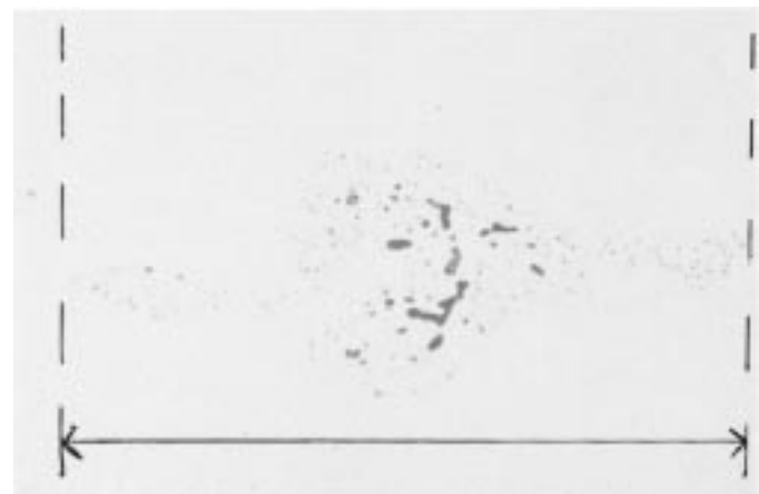
FIG. 3 Example of a spotty oxide inclusion. The maximum Feret's diameter is indicated.
