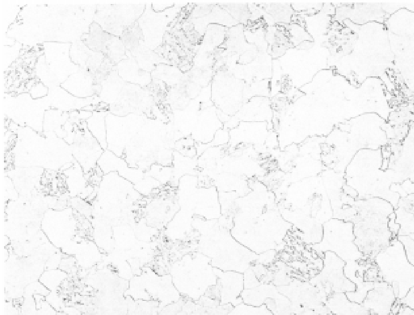
FIG. 1 Example of Replica Microstructure at 100\times LM. Material: See Specification A 335/A 335M, Grade P22. Etchant: 2 % Nital
