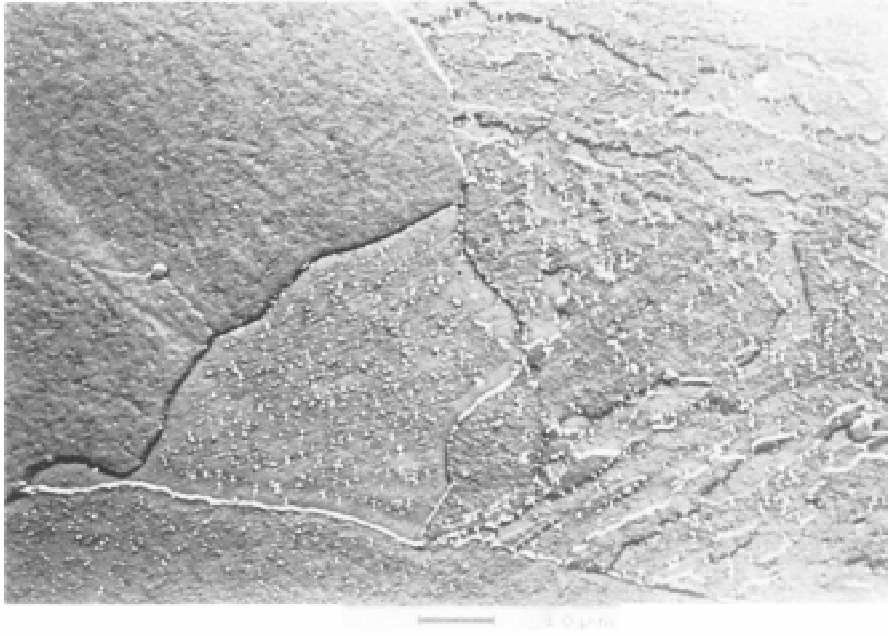
FIG. 4 Example of Replica Microstructure at 1000× SEM. Material: See Specification A 335/A 335M, Grade P22. Etchant: 2 % Nital
