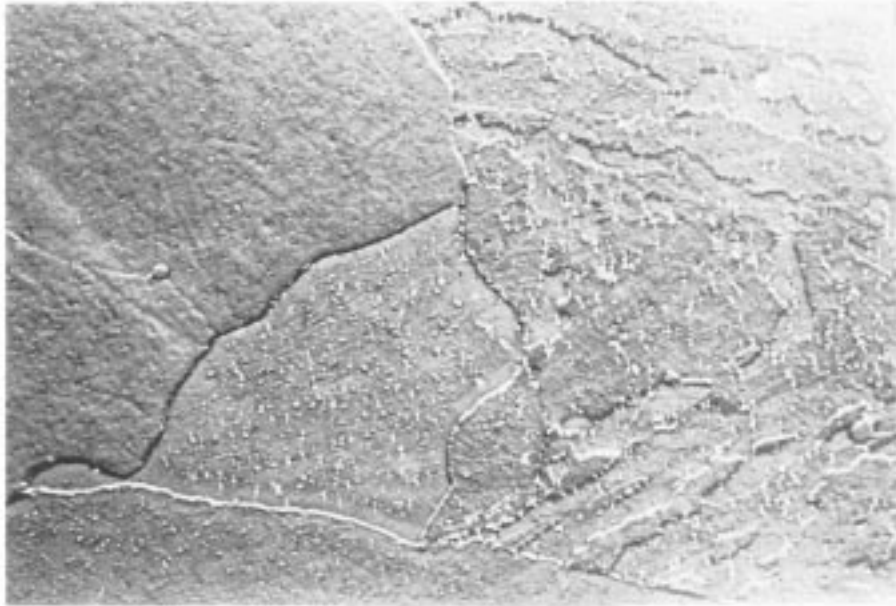
FIG. 4 Example of Replica Microstructure at 1000× SEM. Material: See Specification A 335/A 335M, Grade P22. Etchant: 2 % Nital
