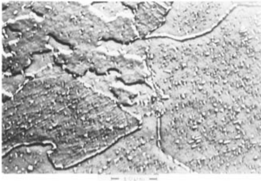
FIG. 5 Example of Replica Microstructure at 2000× SEM. Material: See Specification A 335/A 335M, Grade P22. Etchant: 2 % Nital
