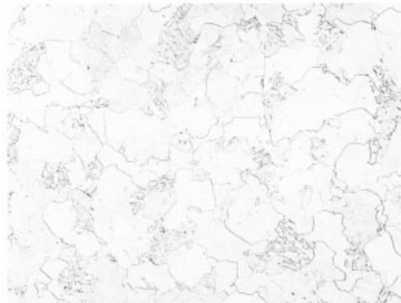
FIG. 1 Example of Replica Microstructure at 100× LM. Material: See Specification A 335/A 335M, Grade P22. Etchant: 2 % Nital
