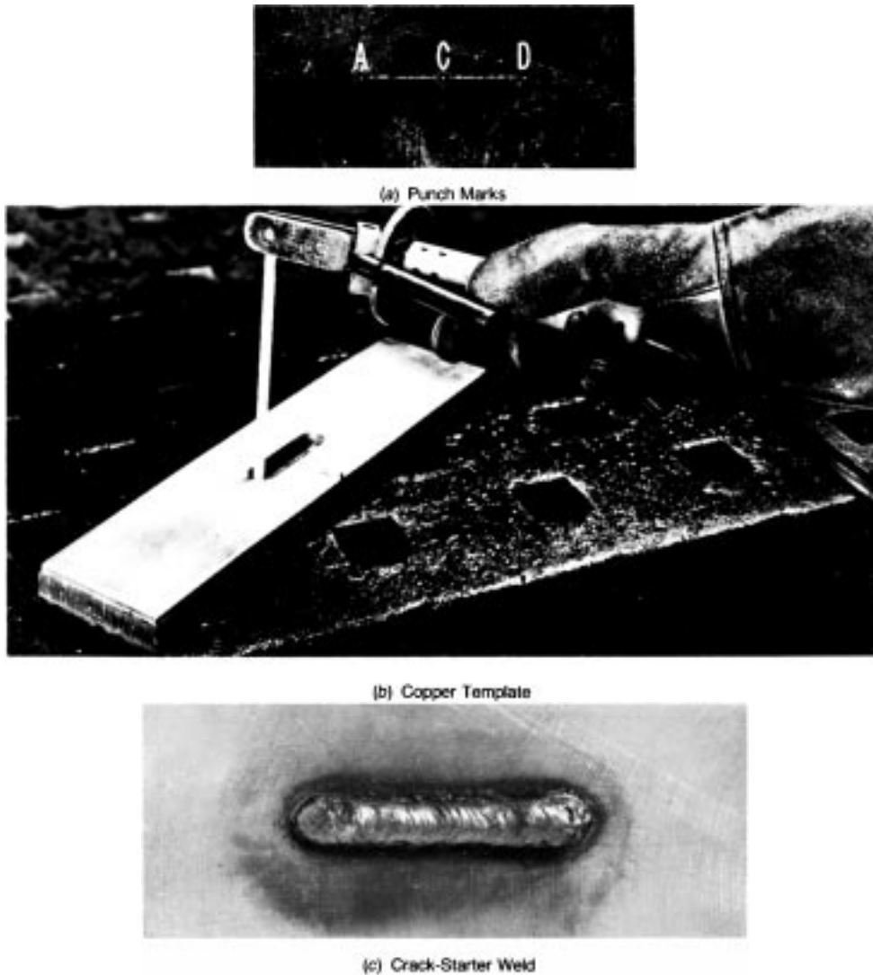
FIG. 7 Methods of Locating the Weld Deposit Properly on the Test Specimen
