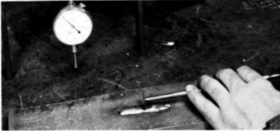
FIG. 8 Notching of Crack-Starter Weld Deposit
