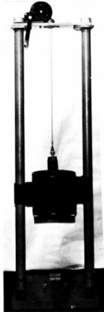
FIG. 5 Portable Drop-Weight Test Machine Used for Tests at Different Fabrication Sites
