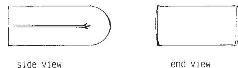
Flattened bend - collapsed eye of the bend
