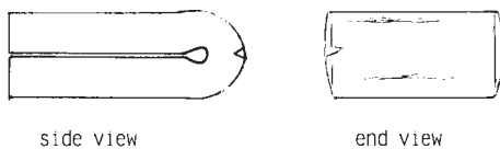
Flattened bend - outer surface and edge cracks
