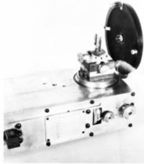
FIG. 2 Universal Camera With Goniometer Head for Back-Reflection Laue Studies
