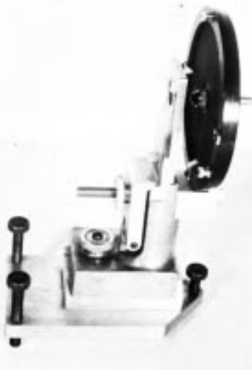
FIG. 1 Back-Reflection Laue Camera for Metallic Sheet Specimens
