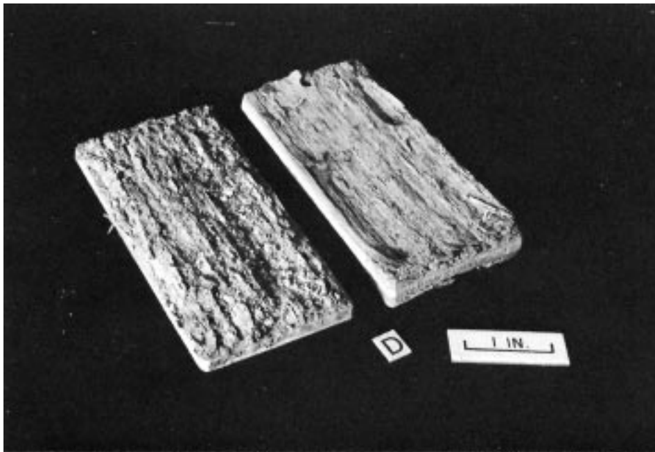
FIG. 6 Examples of Exfoliation Rating ED (Very Severe) (Similar to EC Except for Much Greater Penetration and Loss of Metal)
