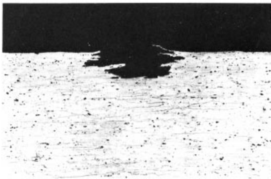
Undermining pitting that may form the surface give the appearance of incipient exfoliation (Keller's Etch; 100X).
