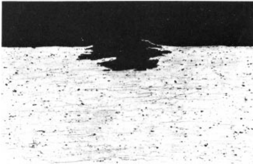
Undermining pitting that may from the surface give the appearance of incipient exfoliation (Keller's Etch; 100×).
