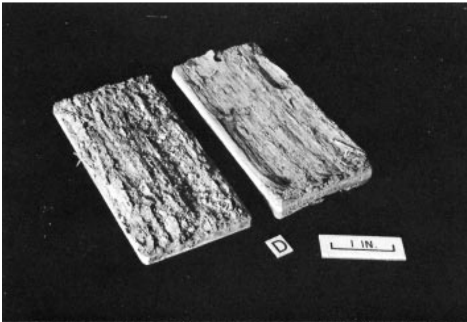
FIG. 4 Examples of Exfoliation Rating ED (Very Severe) (Similar to EC Except for Much Greater Penetration and Loss of Metal)
