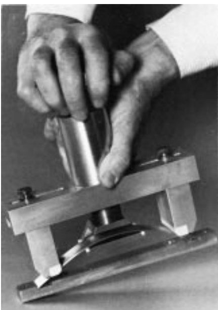
FIG. 2 Stressing Jig and Two-Point Loaded Specimen with Holder (approximately 1/4 actual size)
