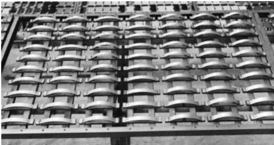
FIG. 4 Bent-Beam Specimens on Atmospheric Exposure Rack
