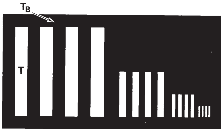
FIG. 1 Targets Used for MRTD Determinations
