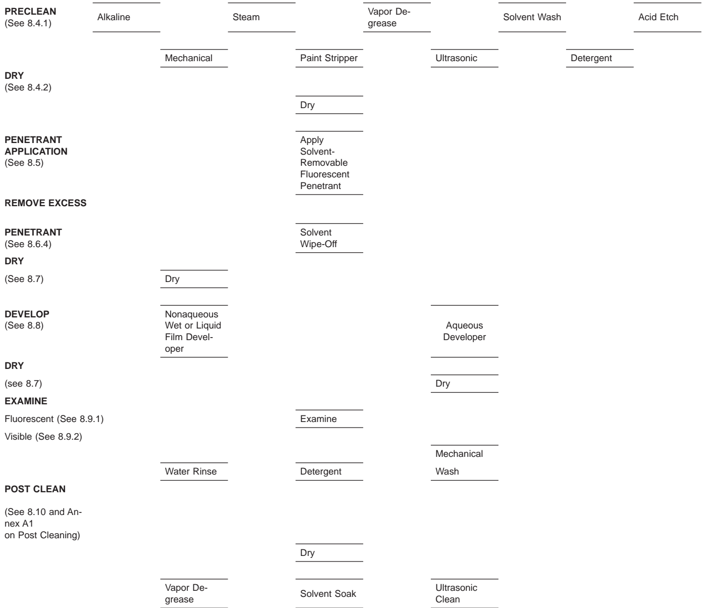
FIG. 3 Solvent-Removable Penetrant Examination General Procedure Flowsheet (Test Method E 1219 for Fluorescent and Test Method E 1220 for Visible Light)
