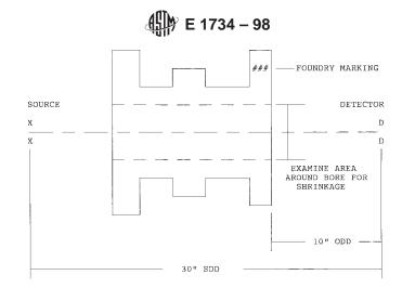
NOTE 1—Indicate scan plan details, including each required view, location of required IQIs and markers, sequence of required views, and direction and maximum speed of manipulation. Where it is impractical to place the IQI on the casting, indicate the selection and location of the appropriate mounting block and IQI.
