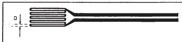
FIG. 2 Typical EMAT Meander Coil for Generation of Surface Waves
