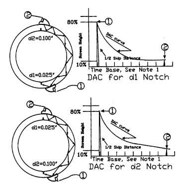
Note1: Time base shall be sufficient in length to display at leaset 1/2 of the cylinder's circumferance. Note2: Drawings of sound paths do not represent the actual number of skip distances. Note3: Drawings are not to Scale.
