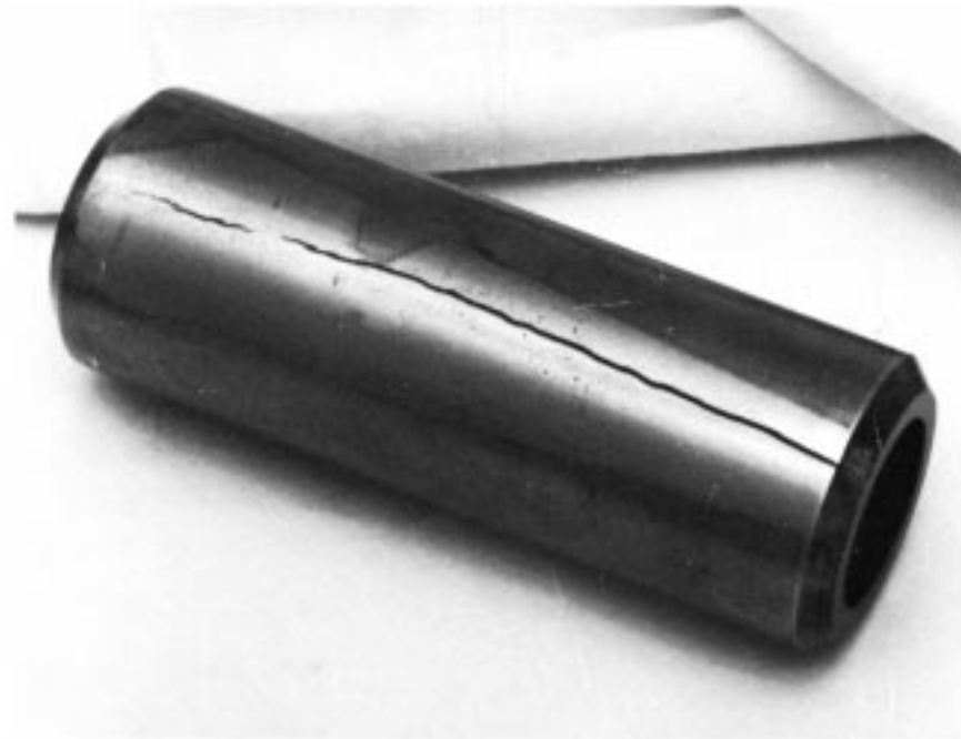
FIG. A1.10 Indications of Surface Cracks (Produced by Circular Indirect Magnetization DC)
