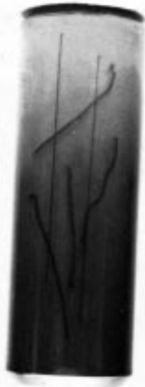
FIG. A1.24 Nonrelevant Indications of Magnetic Writing (Produced by Direct Magnetization, DC Continuous)
