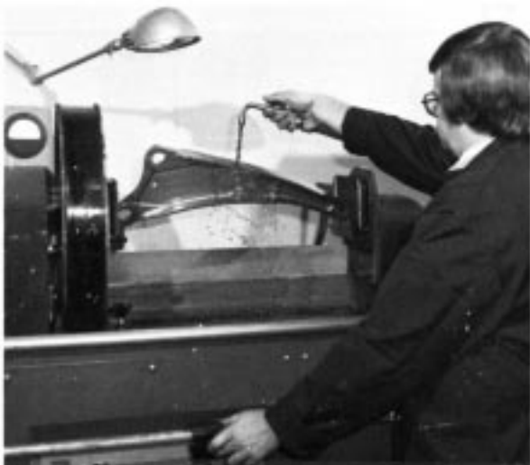
FIG. 5 Direct Contact Magnetization Through Head/Tailstock
