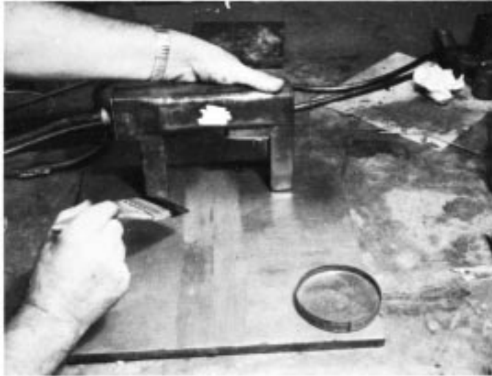
FIG. A1.15 Magnetic Slurry Indications of Surface Cracks in Weldment (Produced by Yoke Magnetization, AC Continuous)
