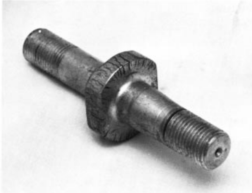
FIG. A1.8 Indications of Surface Cracking (Produced by Circular Direct Magnetization DC Continuous)
