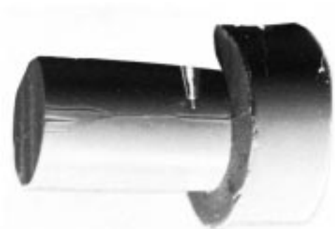
FIG. A1.13 Magnetic Rubber Indications of Surface Cracks in Aircraft Fastener Holes (Produced by Yoke Magnetization DC Continuous)
