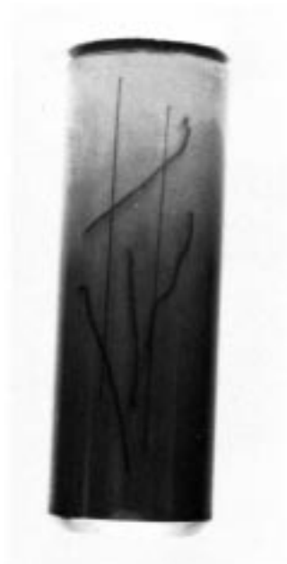
FIG. A1.24 Nonrelevant Indications of Magnetic Writing (Produced by Direct Magnetization, DC Continuous)
