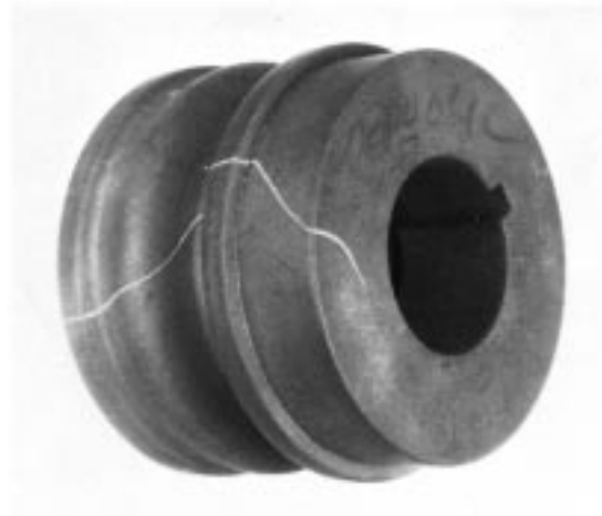
FIG. A1.23 Indications of Surface Cracks (Produced by Central Conductor Magnetization, AC Continuous)
