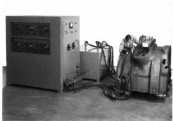
FIG. 6 Direct Contact Overall Magnetization
