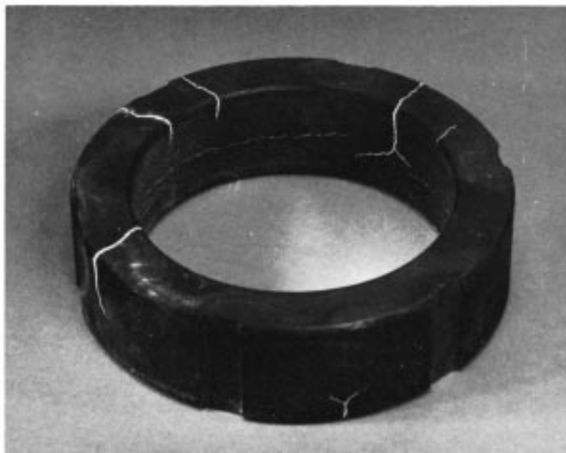
FIG. A1.2 Indications of Surface Cracks (Produced by Central Conductor DC Magnetization)
