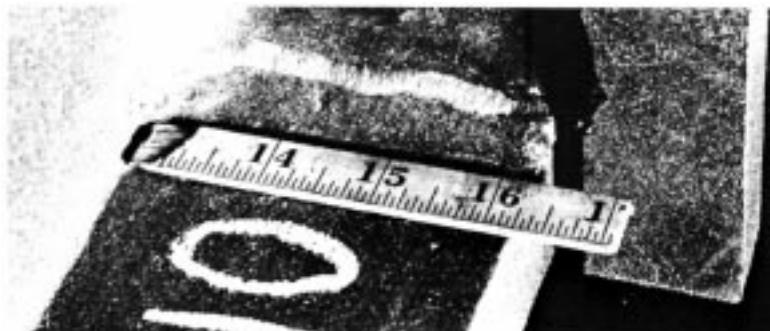
FIG. A1.18 Indications of a Near-Surface Discontinuity (Produced by Prod Magnetization, HWDC Continuous)
