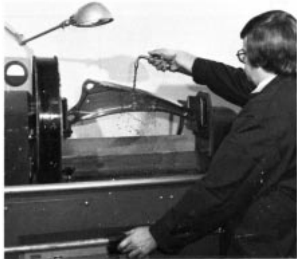
FIG. 5 Direct Contact Magnetization Through Head/Tailstock
