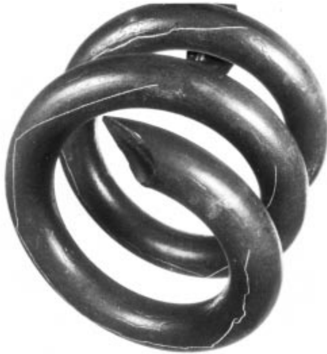
FIG. A1.22 Indications of Surface Cracks (Produced by Circular Direct Magnetization, AC Continuous)
