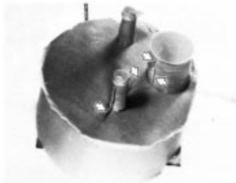
FIG. A1.14 Magnetic Rubber Indications of Surface Cracks in Aircraft Fastener Holes (Produced by Yoke Magnetization DC Continuous)
