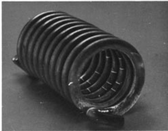
FIG. A1.3 Indications of Surface Cracks (Produced by Central Conductor DC Magnetization)
