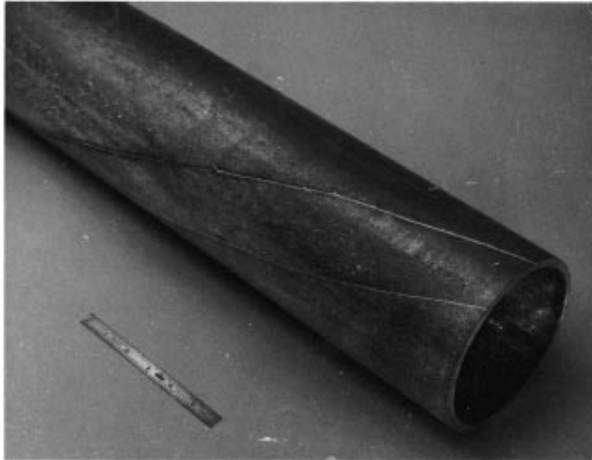
FIG. A1.4 Surface Indications (Produced by Central Conductor DC Magnetization)
