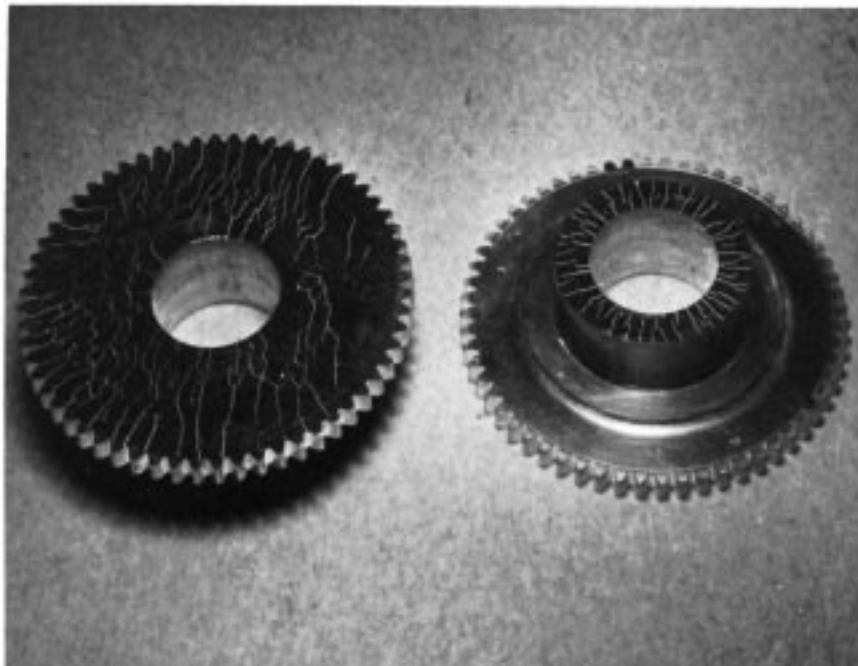
FIG. A1.1 Indications of Surface Cracks (Produced by Central Conductor DC Magnetization)
