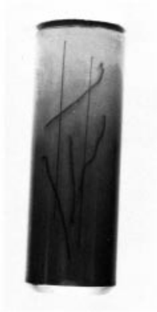
FIG. A1.24 Nonrelevant Indications of Magnetic Writing (Produced by Direct Magnetization, DC Continuous)
