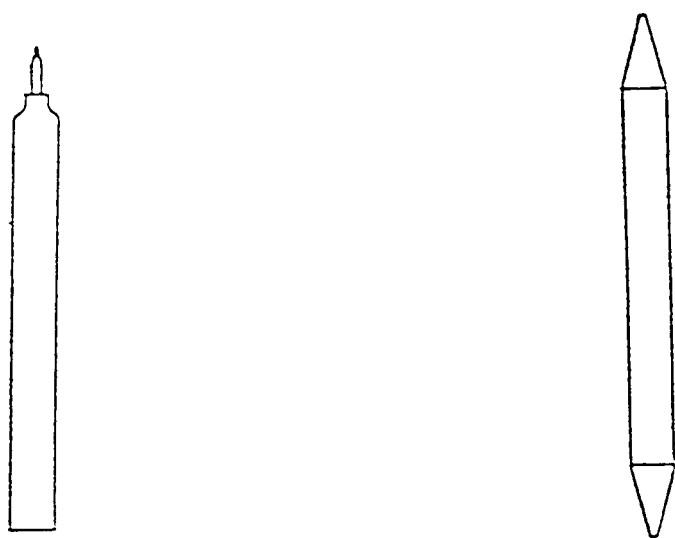
(a) Needle-Point, Thoriated-Tungsten Wire Mounted in Copper Rod (b) Tungsten or Silver Rod with Conical Tip
