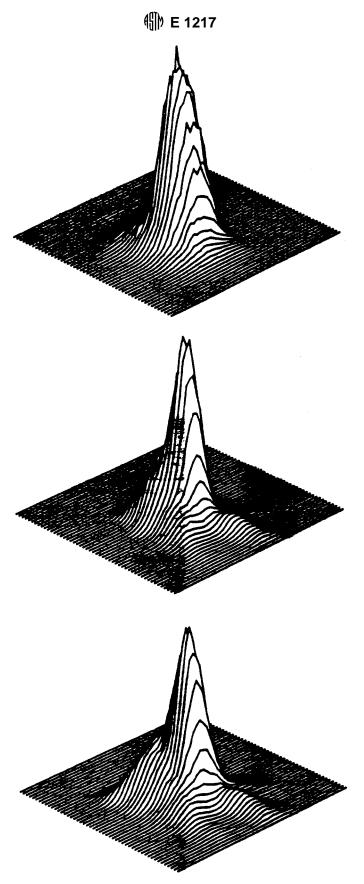
Note 1—Elastic-peak images are for an analyzer pass energy of 50~eV and for electron energies of 100~eV (top), 500~eV (center), and 1000~eV (bottom). The horizontal distance scanned by the electron beam on the specimen (corresponding to the bottom left to right line scan in each image) was 13~mm and the vertical distance was 15~mm.
