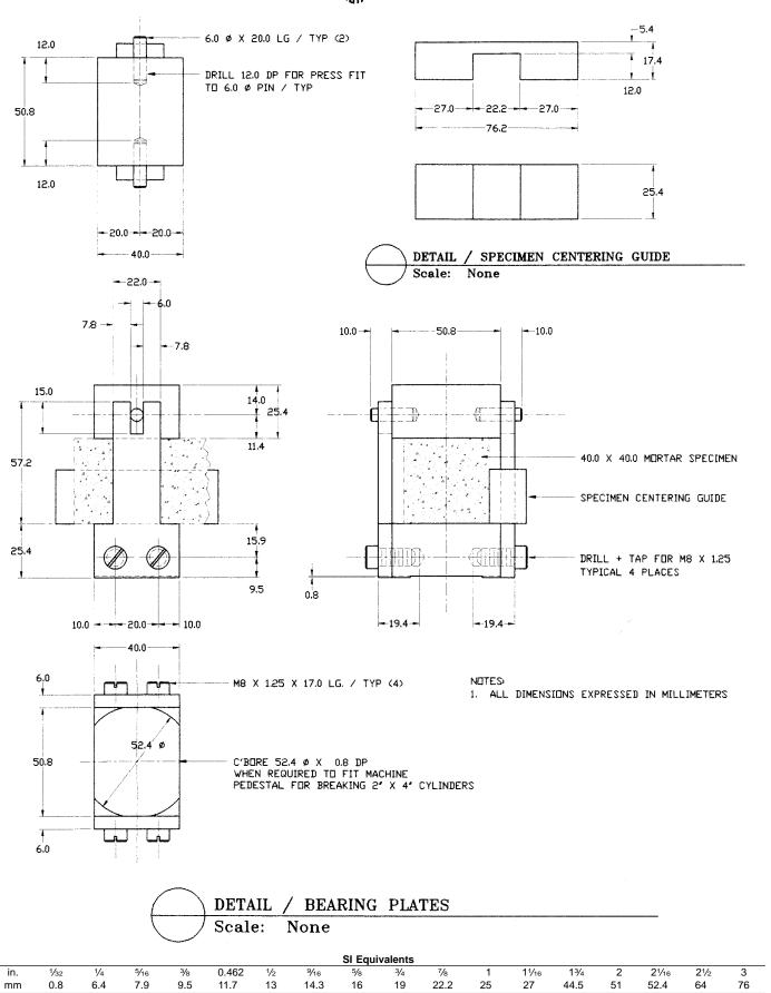
FIG. 1 Bearing Plates and Bearing Plate Aligning Device for Testing 40 by 40 by 160-mm Mortar Prisms as Modified Cubes
