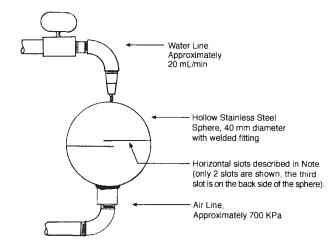
Note 1—Cut three horizontal air slots around circumference of hollow sphere using a 0.20 mm thick diamond lapidary saw covering 120° to 150° each and spaced approximately 5 mm apart. Air passing through these slots strikes the water (which is flowing over the outer surface of the sphere) to produce a spray.
