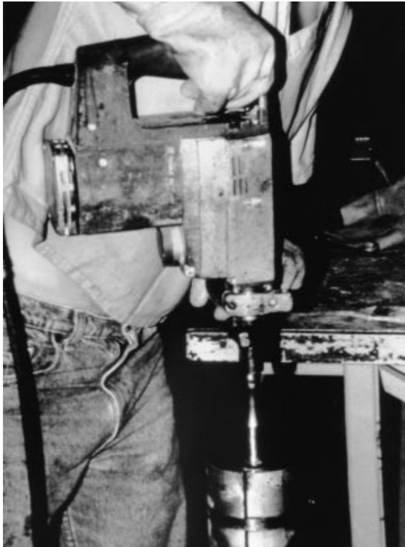
FIG. 1 Vibrating Hammer for Molding RCC Samples
